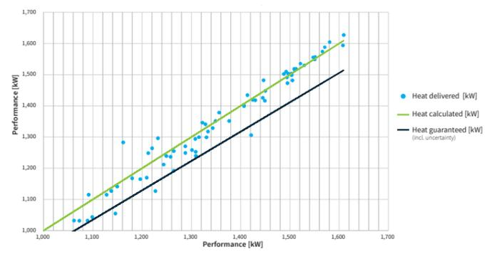
Solar field performance (measured vs. calculated vs. guaranteed) based on plant monitoring between 11 May - 20 June, 2017
