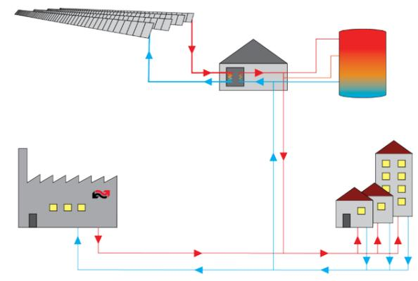
The solar plant consists of 13 rows of flat solar-thermal panels with up to 20 collectors in each row. The 13,3m<sup>2</sup> optimized panels have shown the highest performance among all known mass-produced large-scale collectors on the market. They also come with a 10-year warranty setting a new standard on the long-term quality and reliability of solar systems.
